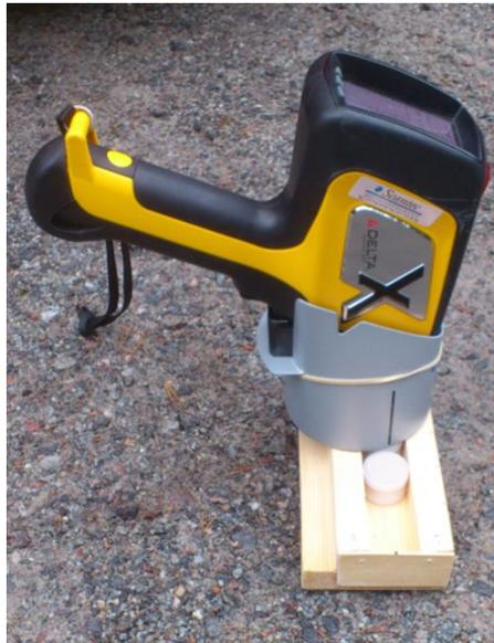
**Figure 2 The FPXRF Delta 50 performing a NIST check in a field environment**
