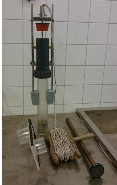
**Figure 12 Kajak sediment sampler together with the plastic slicing tool**
