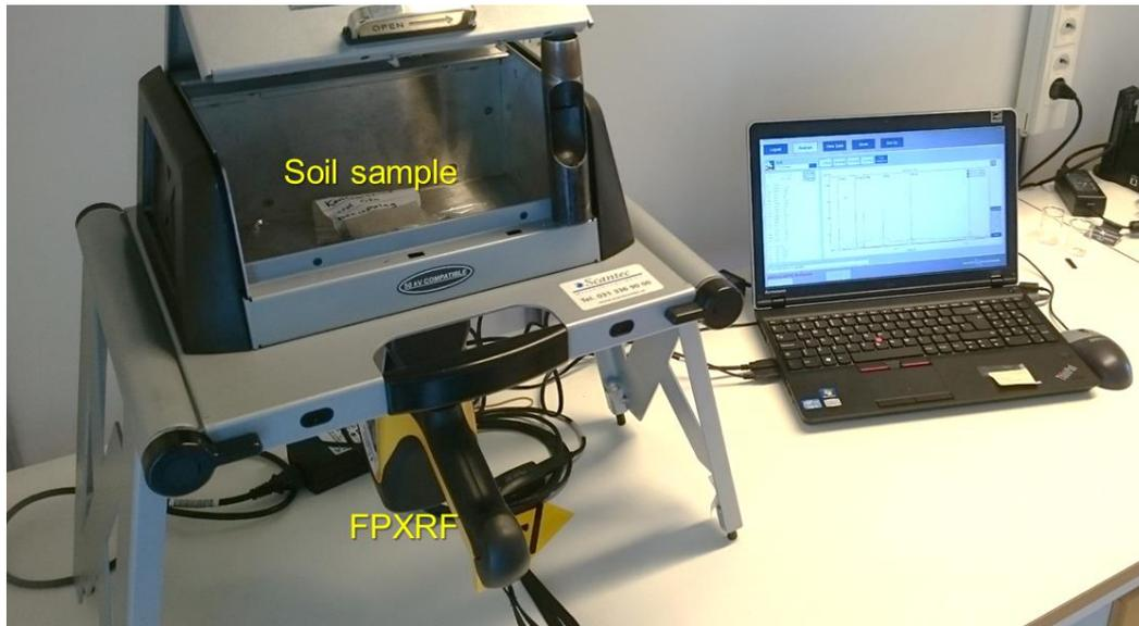
**Figure 3** FPXRF work station in a lab environment. A soil sample in a zip bag is situated on top of the FPXRF measuring aperture window in the shielded enclosure.
