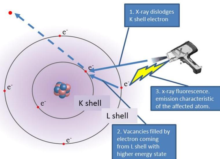
**Figure 1** When the X-rays emitted from the FPXRF enter the atom structure electrons in the inner shells can be dislodged. The vacant spot will be filled with an electron from an outer shell. As that electrons has a higher energy level the energy balance is disrupted. In order to restore the energy level a photon is sent out with a distinct energy spectra for each metal.
