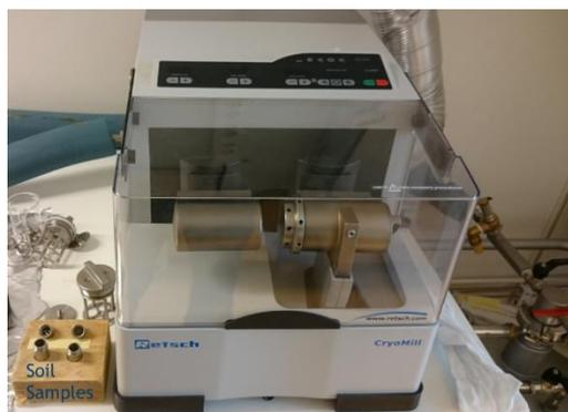
**Figure 10 Cryomill grinder with the small metal soil sample containers to the left. To the right are the connection pipes to the nitrogen tank.**
