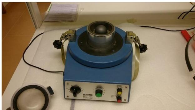
Figure 11 FRITSCH Pulverisette grinder. Soil sample is in the top container with one large metal ball.
