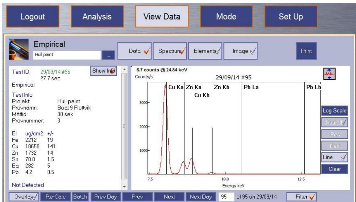
**Figure 5 Example of FPXRF presentation on a lab PC. In the left window the contamination load in  $\mu\text{g}/\text{cm}^2$  is presented in a similar way as on the FPXRF in the field. In the right hand window the spectrum response is presented in Counts/s as a function of the energy in keV. In the left hand table the Cu, Zn, Pb and Sn content is presented**
